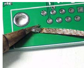
Using solder wick to remove excess solder
